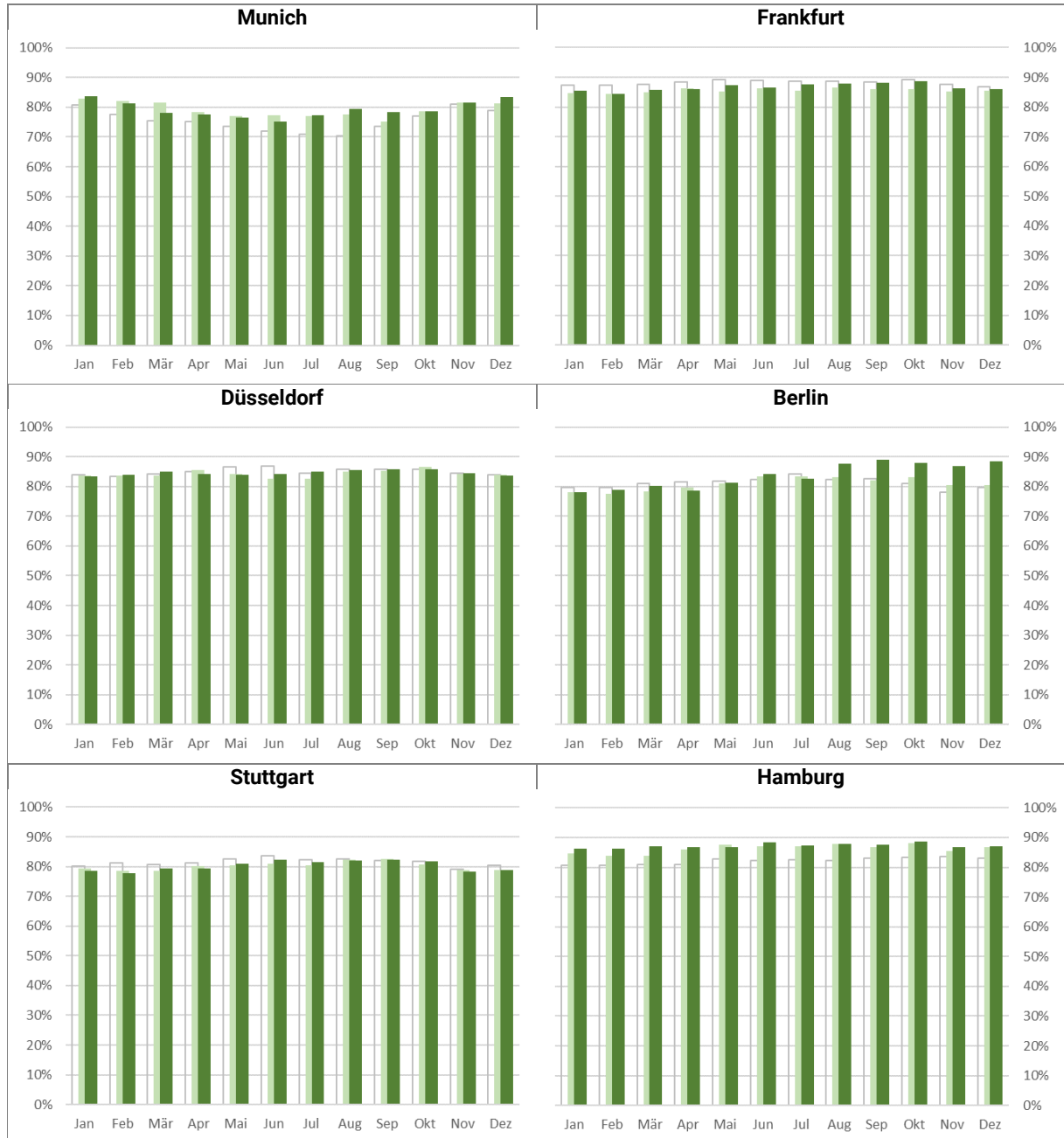
Fig. 9: Average Prognosis score of all TOBT updates per month compared to the same month in the previous year (light green) and 2019 (white).
